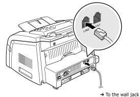
**2** To connect a telephone and/or answering machine to your machine, plug the cord of your extension phone or answering machine into the **EXT** jack.
